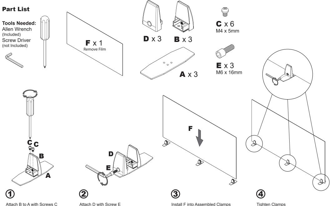
Install F into Assembled Clamps
